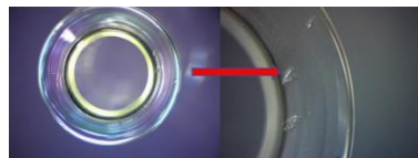
Figure 14 Cracks in the glass
